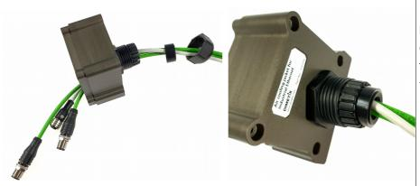
Insert the cables into the cable gland of the rear cover.
